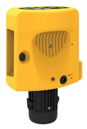
The removable Compression Module contains all the active components of the Lifeline ARM device system, including the User Control Panel, Battery Pack, and Compression Piston. It also houses a software-controlled motor that controls both the rate and depth of compressions.
